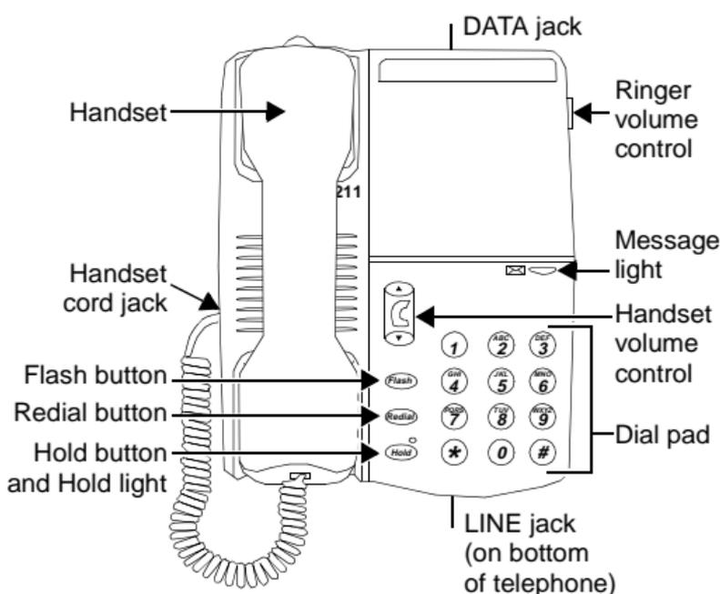
**Figure 1. The 6211 Telephone, Top View**
